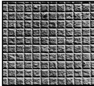
To calculate the electron microscope magnification using the pattern of the diffraction grating replica:
